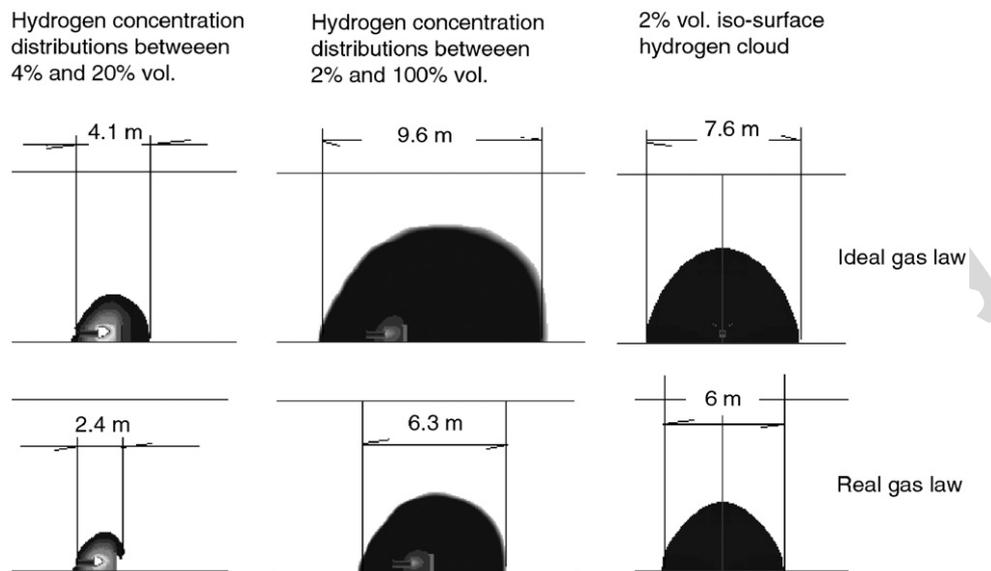
Fig. 6. Hydrogen cloud 5 s after the onset of release using ideal gas law and real gas law. Top three pictures: ideal gas law. Bottom three pictures: real gas law. Left: hydrogen concentration distributions between 4% and 20% vol on the plane that is in the direction of the release. Middle: hydrogen concentration distributions between 2% and 100% vol on the plane that is in the direction of the release. Right: 2% vol of hydrogen cloud iso-surface viewed in the direction of the release.
