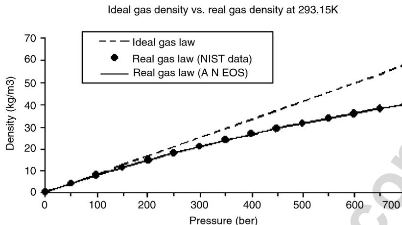
Fig. 2. Density deviation from ideal gas law as a function of pressure at 293.15 K. At 700 bar, the real gas density is about  $40 \text{ kg/m}^3$  but is overestimated by 45% when using the ideal gas law. Solid line: ideal gas law. Dots: NIST data [7]. Dash line: real gas law using AN-EOS.
