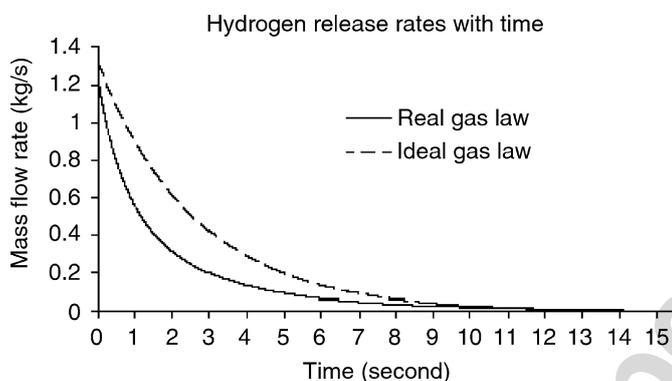
Fig. 3. Choked hydrogen release rate for the impingement release. Initial tank pressure: 700 bar. The leak orifice size:  $\frac{1}{4}$ ". Solid line: the choked release rate with using real gas properties (The predicted choked release lasts 14.14 s). Dash line: the choked release using ideal gas law (The predicted choked release lasts 15.45 s). The ideal gas law overestimates the hydrogen release rate by up to 53% 3 s after the onset of the release.
